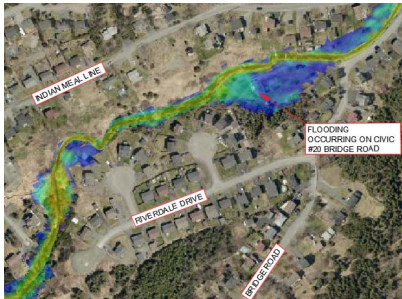
Figure 19: Flooding Occurring on Civic #20 Bridge Road 100 Yr – 2 Hr CC
