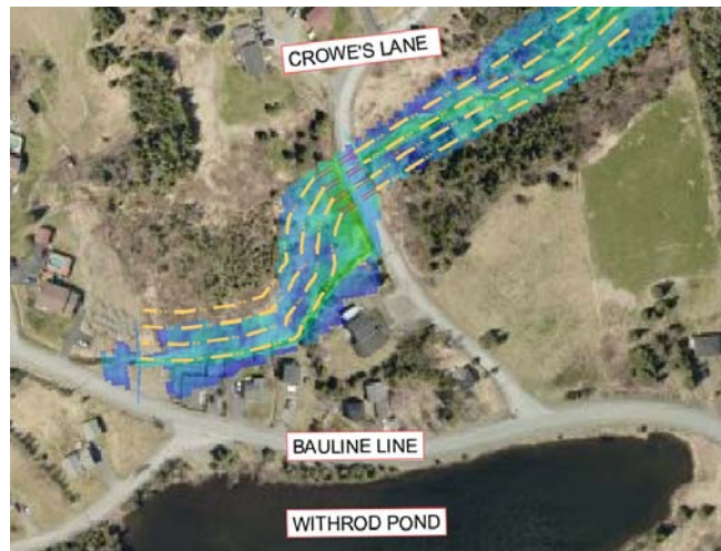
Figure 27: Flooding Occurring on Crowe's Lane 100 Yr - 24 Hr CC
