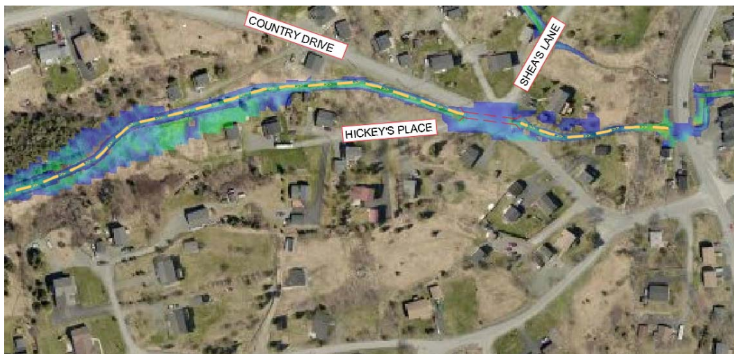
Figure 23: Flooding Occurring Near Hickey's Lane, Intersection of Country Drive/Hickey's Lane 100 Yr - 24 Hr CC
