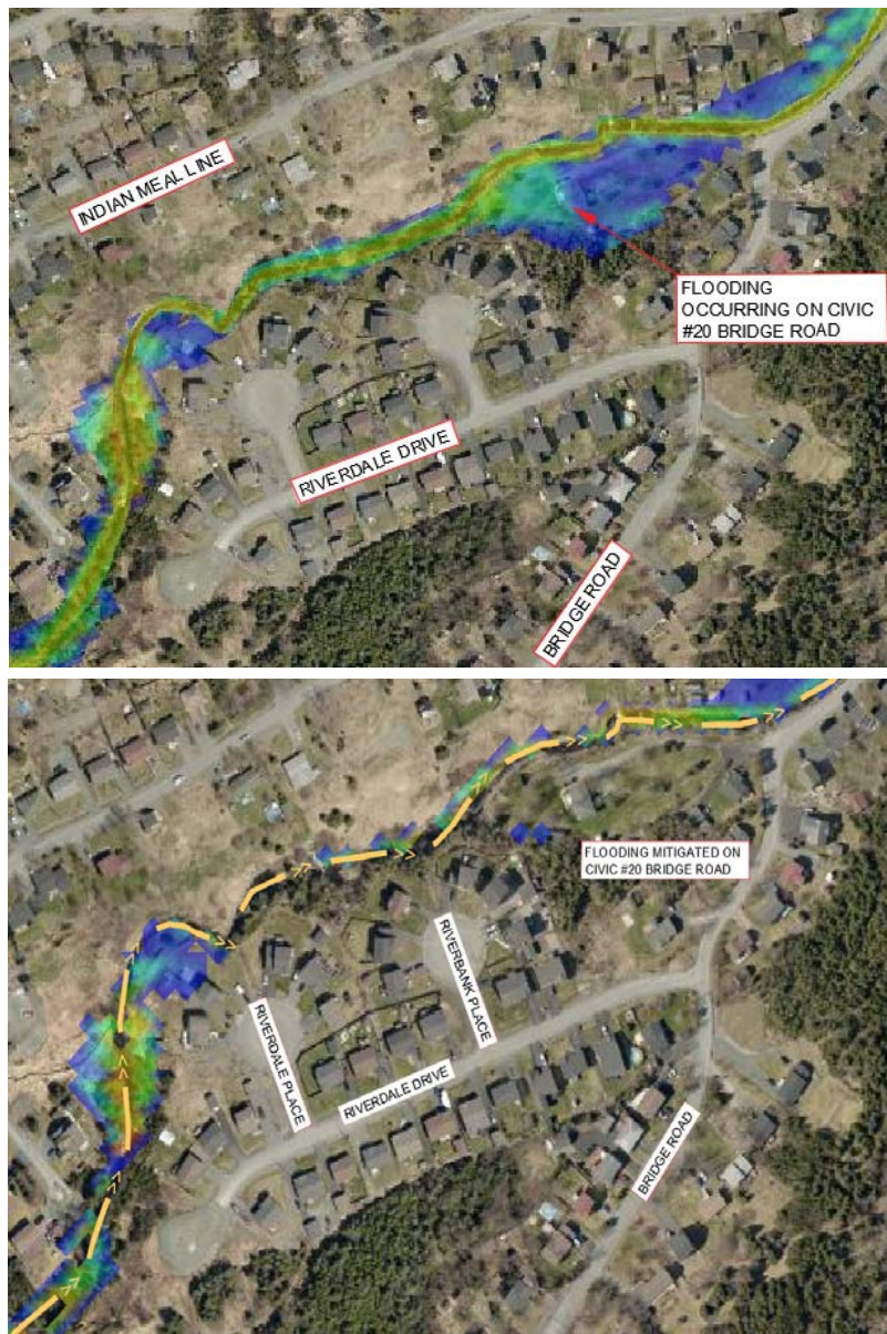
Figure 42: Bridge Road Before Upgrades vs Bridge Road After Upgrades
