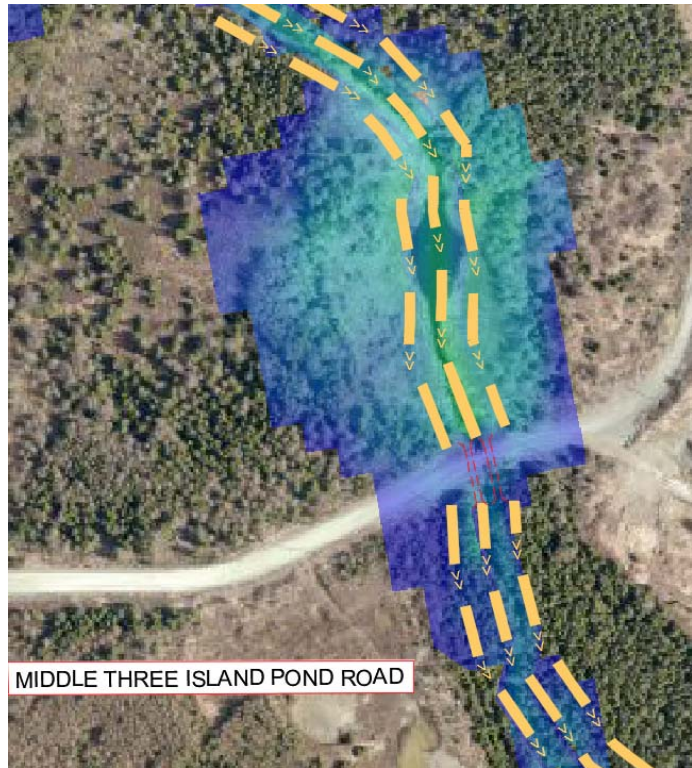
Figure 13: Flooding Occurring on 100 Yr – 6 Hr CC
